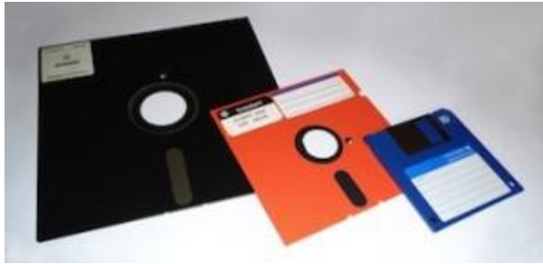
Figure 14 Floppy-disk evolution (8" to 5 1/4" to 3 1/2") (Public Domain)
