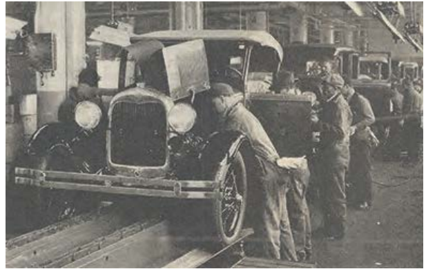
Figure 63 In this image from a 1928 Literary Digest interview with Henry Ford, workers on an assembly line produce new models of Ford automobiles.
