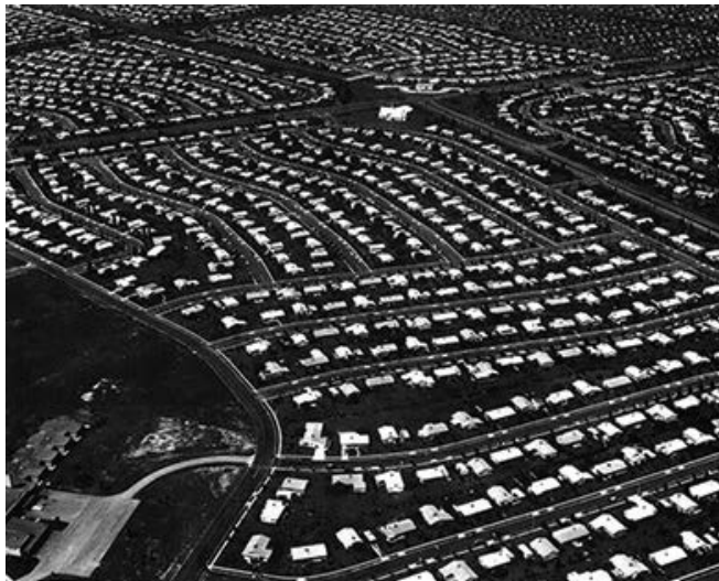
Figure 141 This aerial view of Levittown, Pennsylvania, reveals acres of standardized homes. The roads were curved to prevent cars from speeding through the residential community that was home to many young families.
